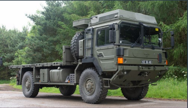
MAN HX60 6x6 Cargo (Medium) Medium Mobility 6 Tonne - Flatbed
