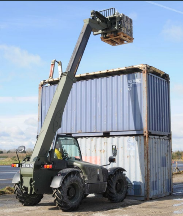
JCB 541-70 (medium) The side mounted JCB provides instant steering selection between all wheel steer, front wheel steer and crab steer modes ensures ease of operation, a tight turn radius of 3.7 metres gives greater manoeuvrability. Forward reach of 3.7 metres, lift capacity 4.1 tonnes and lift height of 7 metres.
