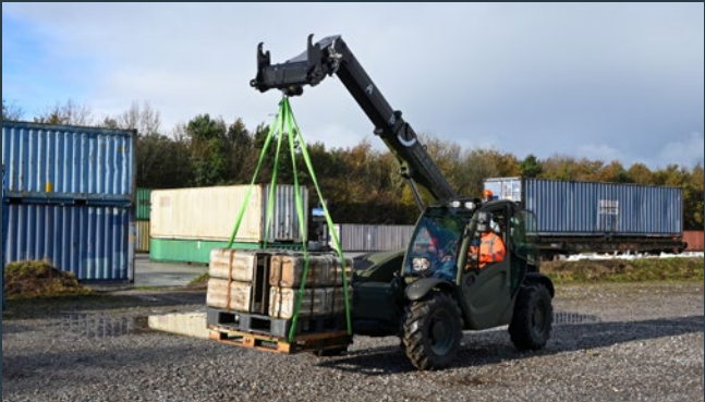
Manitou MT625H 4 equal sized wheels enhance tractive effort to give excellent loader performance. In addition, flotation over soft ground conditions and ground clearance are first class. Permanent 4 wheel steer, together with the compact machine size, means an exceptionally tight turning circle with a radius of just 3 metres for great manoeuvrability and handling in small areas.
