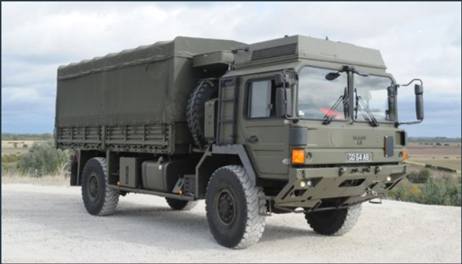
MAN HX60 4x4 Cargo (Light) Medium Mobility 6 Tonne - Canopy
