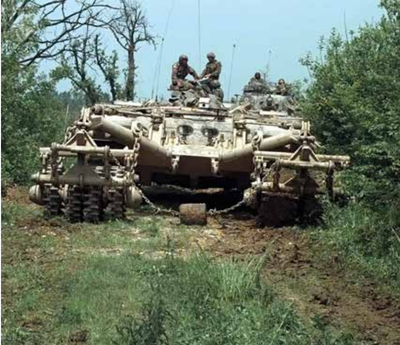
A remotely controlled Panther armored mine clearing vehicle leads a column of armored vehicles down a road near McGovern Base, in Bosnia and Herzegovina on May 16, 1996, during Operation Joint Endeavor. The Panther, based on a modified M-60 tank hull, uses metal rollers to set off contact or magnetic mines. The Panther is being operated by the 23rd Engineer Battalion, 1st Brigade, 1st Armored Division. DoD photo by Staff Sgt. Jon Long, U.S. Army, Released
