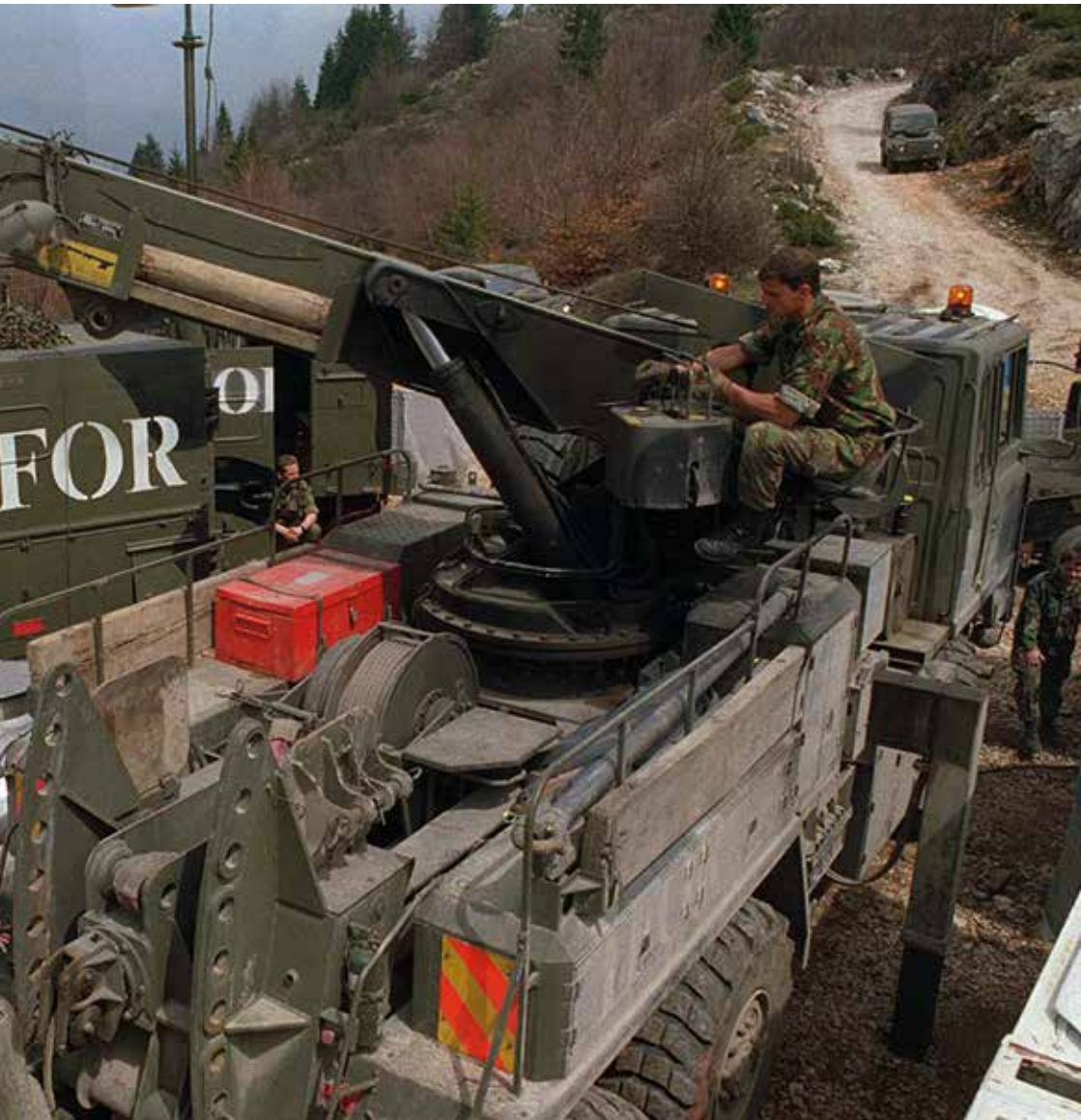
A British Army Corporal manoeuvres the jib of the Recovery Vehicle as one of his team prepares to hook on a water tank. The tank will improve conditions for the signalers manning a rebroadcast site on Trebevic Mountain overlooking Sarajevo. Photo: Sergeant Dave Whitley, Crown Copyright
