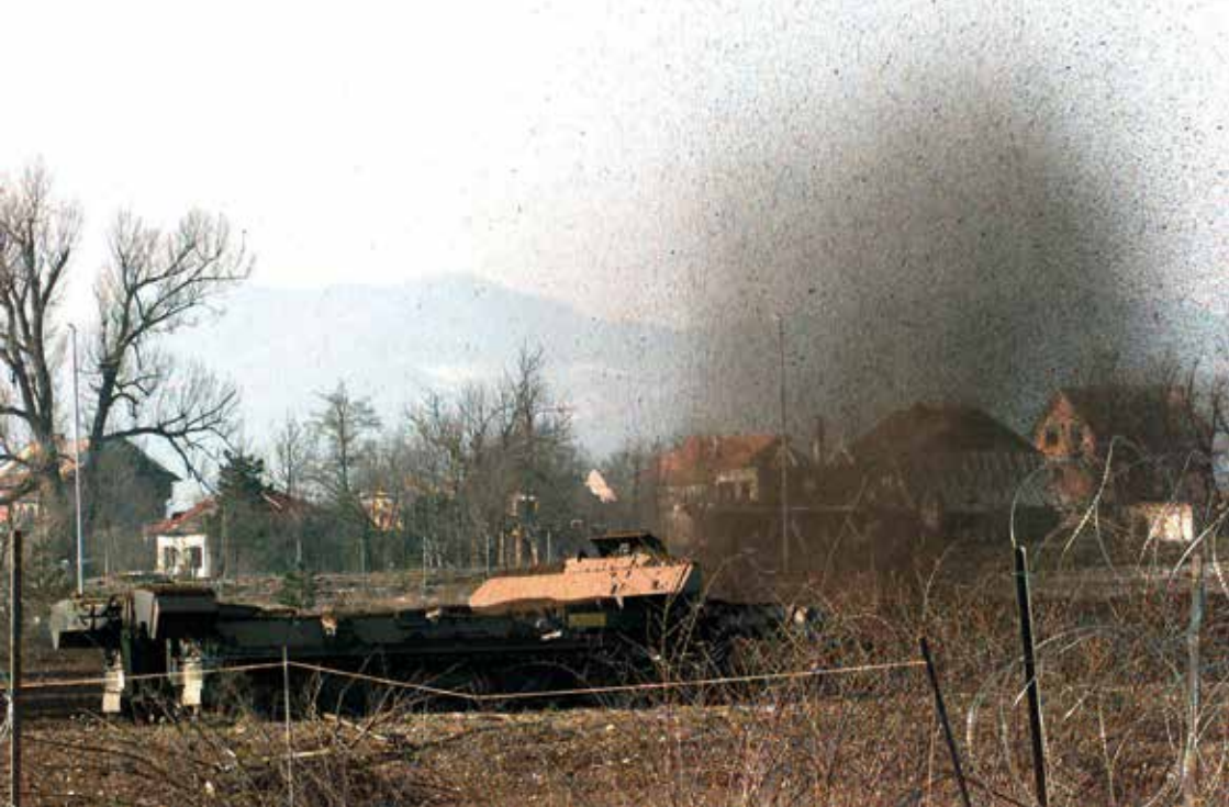
A German Army Armored Mineclearing Vehicle, attached to the Joint German-French Engineering Brigade, is used to clear a field of possible mines in Butmire, Bosnia-Herzegovina, which will later be used to house NATO troops. Photo: Charles L Withrow, US Department of Defence, Wikimedia, Released
