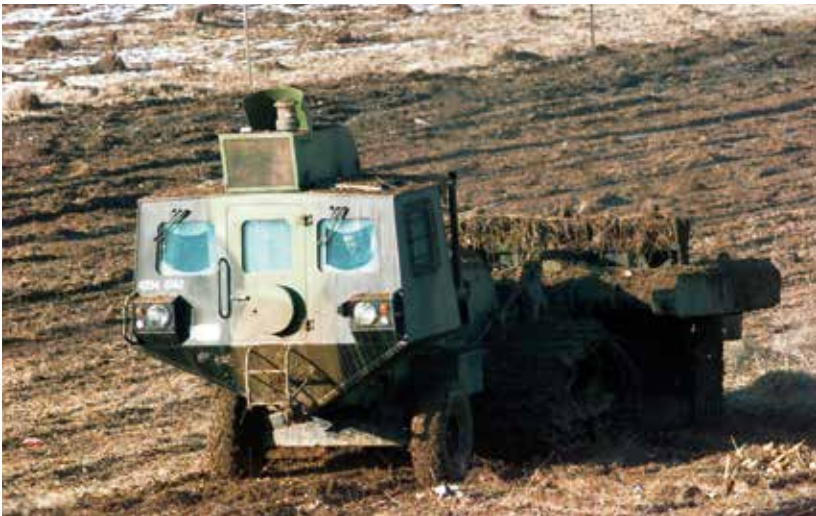
A French Army 17th Engineering Regiment Aardvark Joint Services Flail Unit (JSFU) is used to clear a possible mine field in Butmir, Bosnia-Herzegovina during Operation Joint Endeavor. Photo PHAN Charles L Withrow, US Department of Defence, Wikimedia, Released
