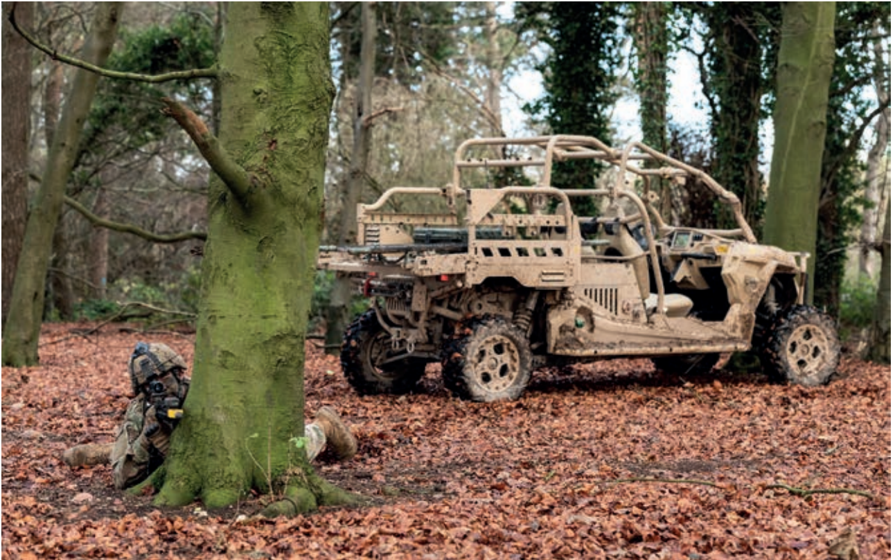
Pictured is the MRZR X, a modular multi-mission support mobility platform that has multiple modes of working from operator driving to autonomous operation. Photo: Corporal Rebecca Brown, Crown Copyright
