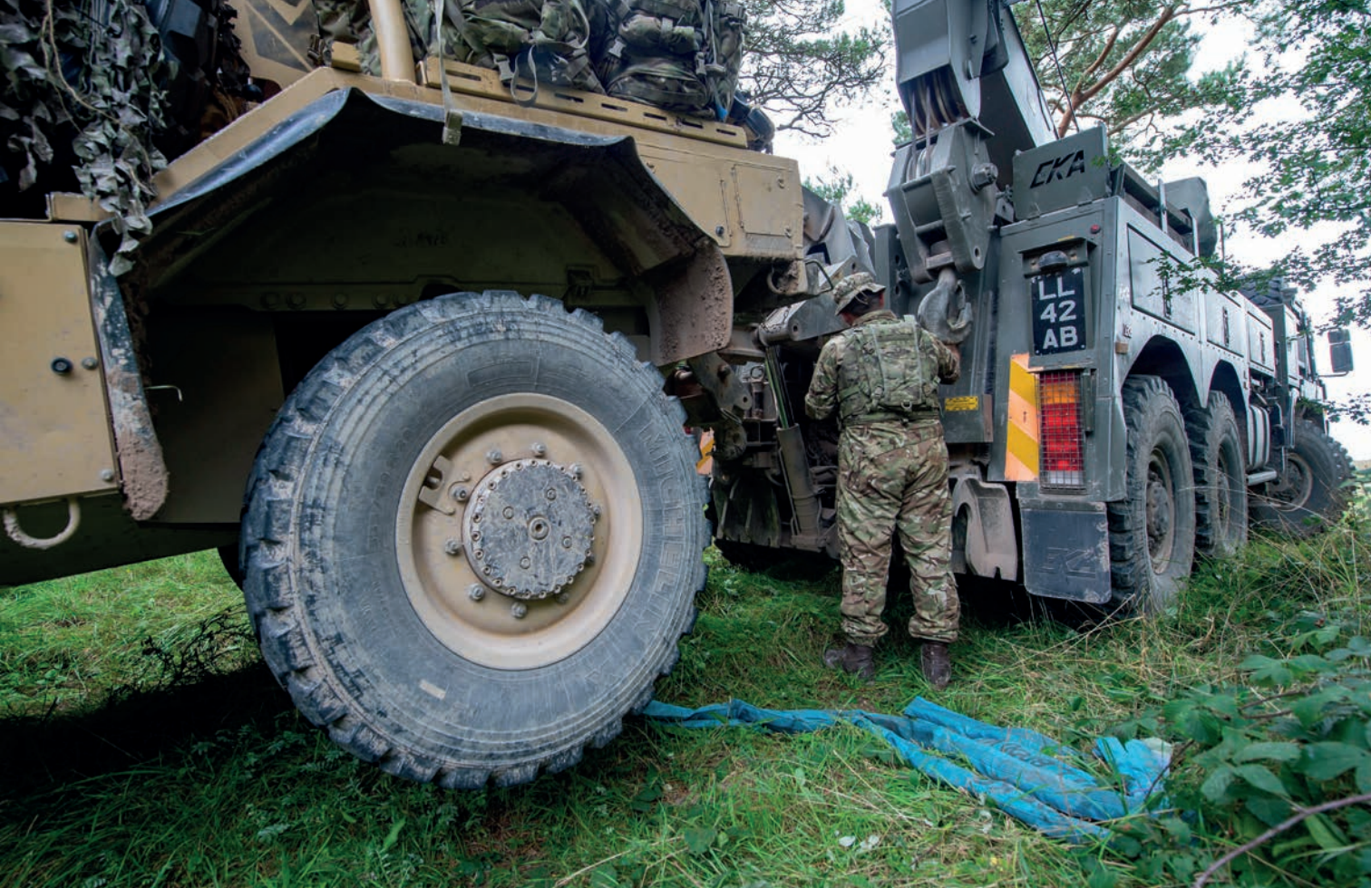
A Recovery Mechanic from the Royal Electrical and Mechanical Engineers (REME) lifting the rear end of a Jackal in preparation to recover the vehicle. Army Reserves from 103 Battalion REME training in the UK before deploying to Poland as part the UK's commitment to NATO enhanced Forward Presence (eFP) in Eastern Europe. Photo: Corporal Simon Lucas, Crown Copyright
