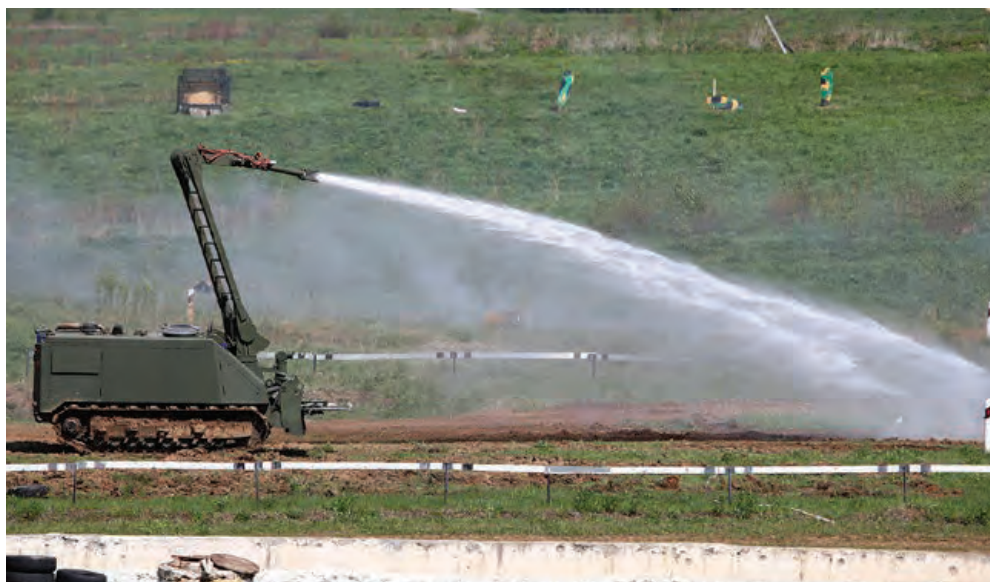
Pictured is the Uran-14 Firefighting Unmanned Ground Vehicle during the scientific and technical forum of The Day of Advanced Technologies of Law Enforcement Authorities of the Russian Federation. Photo: Vitaly V. Kuzman, Creative Commons Attribution-NonCommercial-NoDerivatives 4.0 International License, https://www.vitalykuzmin.net/
