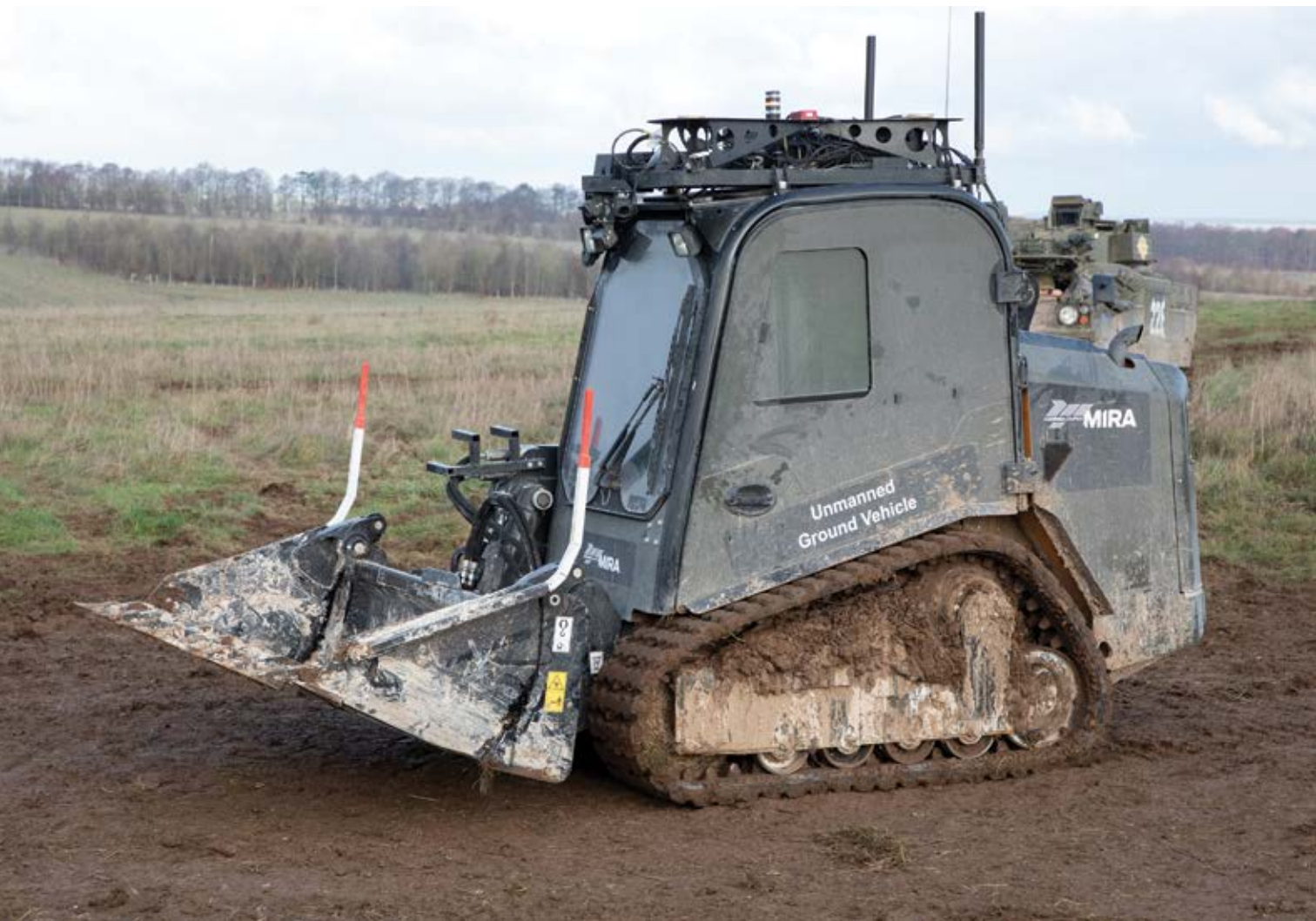
Pictured is an unmanned Compact Track Loader fitted with a MIRA Modular Autonomous Control Equipment (MACE). Photo: Sergeant Peter George, Crown Copyright
