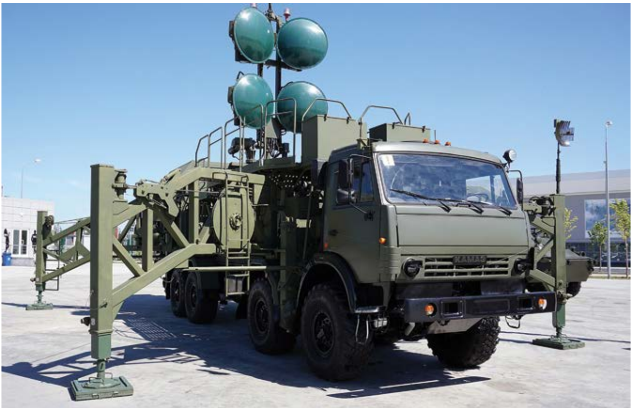
Pictured is a Russian R-431AM antenna module of Redut-2US signal and communications system at the Military-technical forum ARMY-2018 at the Park Patriot in Russia. Photo: Vitaly V. Kuzmin, www.vitalykuzmin.net , Creative Commons Attribution-NonCommercial-NoDerivatives 4.0 International License
