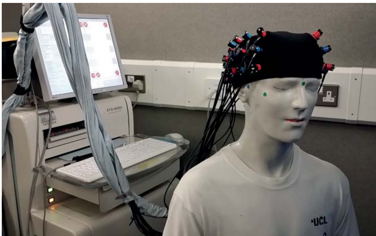
Pictured is a functional near-infrared spectroscopy (fNIRS) by Hitachi. Image: Walej, UCL Speech, Hearing and Phonetic Sciences, Creative Commons Attribution-Share Alike 4.0 International License, Wikimedia
